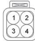
E27: Harness plug (to power harness)
